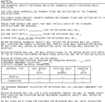
$\bar{\rm D}{\rm O}$  not place no.57 stone for footings for retaining wall no. Until excavation  $\bar{\rm D}{\rm IMENSIONS}$  and foundation material are approved.
